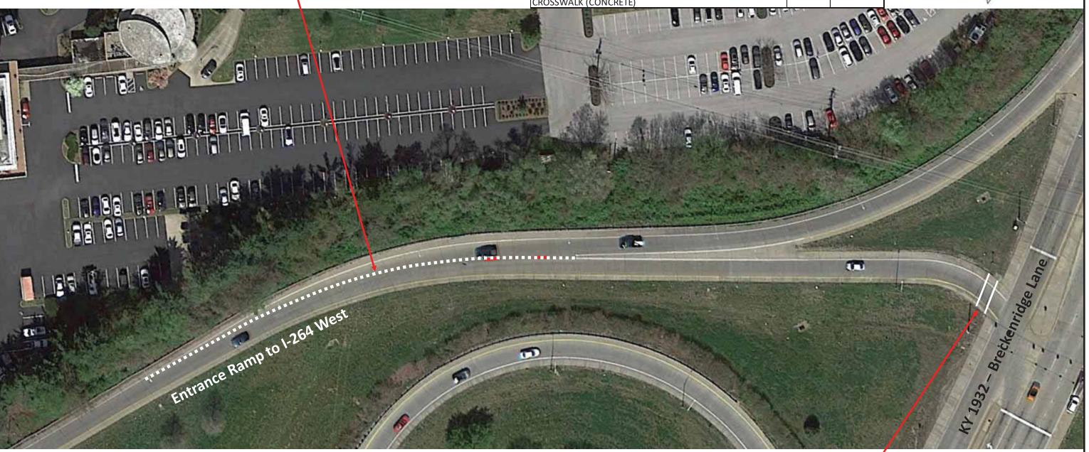
Remove existing markings to refresh 6-inch white HPS-8 crosswalk stripes. Remove edge lines within the limits of the crosswalk.
