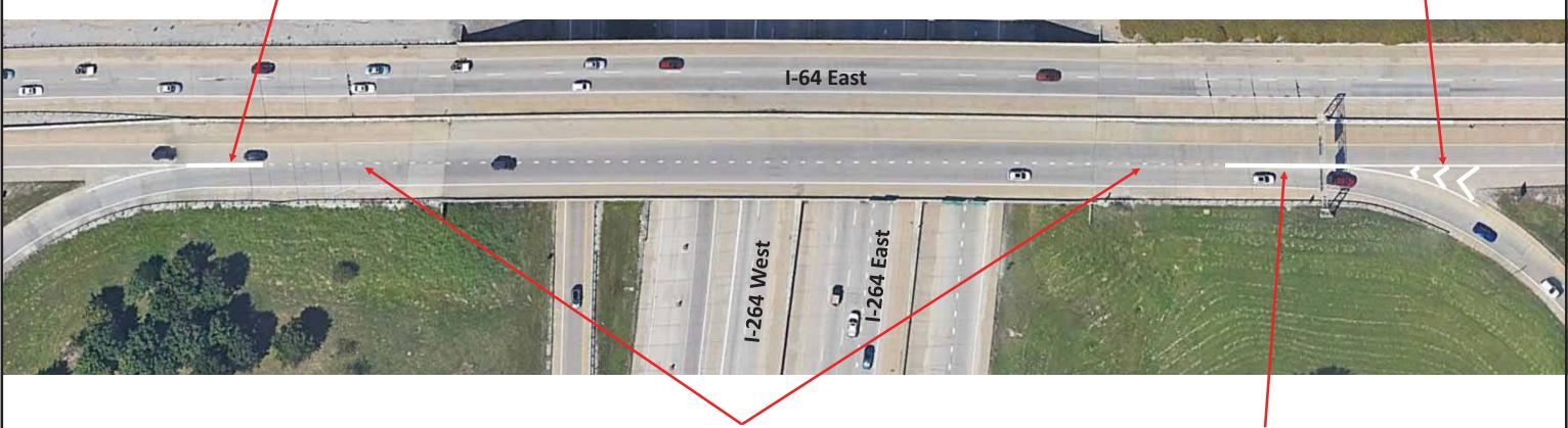
Extend 12-inch solid white painted gore stripe approximately 50' over the existing dotted lane line. Stripe over any old pavement marker castings. Install two coats of paint for all new stripes.
