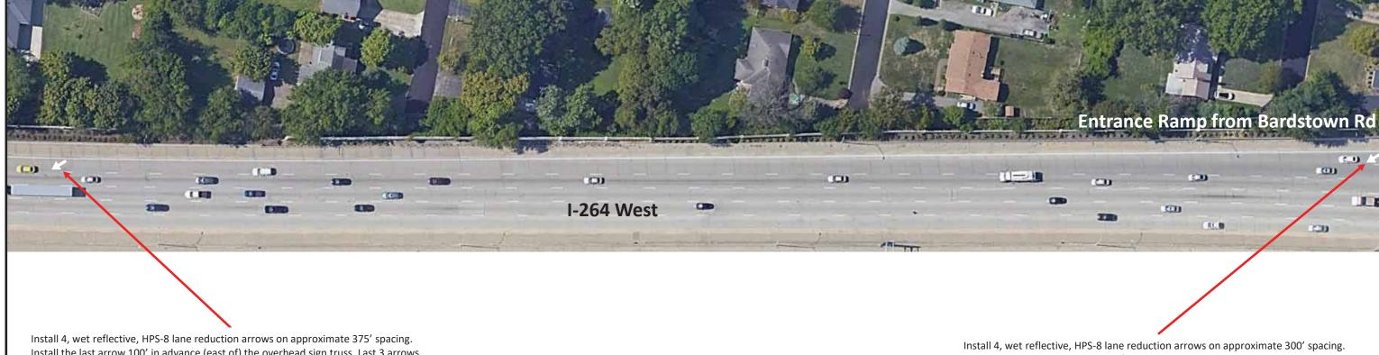
Install 4, wet reflective, HPS-8 lane reduction arrows on approximate 375' spacing. Install the last arrow 100' in advance (east of) the overhead sign truss. Last 3 arrows on next sheet. If possible, avoid pavement joints with minor spacing adjustments.
