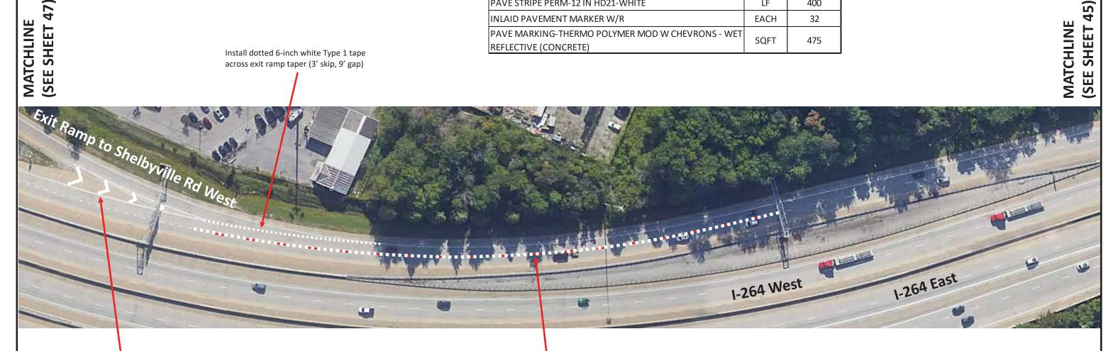
Install 48-inch white, wet reflective, HPS-8 gore chevrons on 40' spacing.
