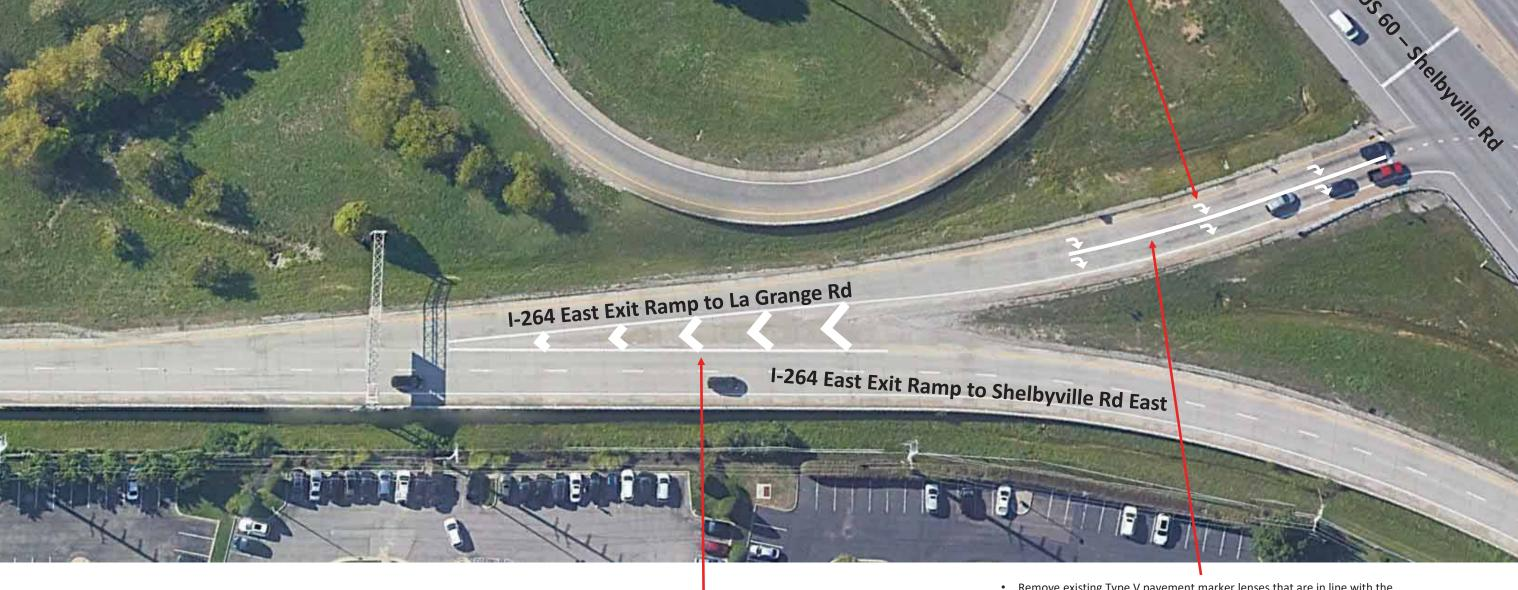
Install 48-inch white, wet reflective, HPS-8 gore chevrons on 40' spacing.
