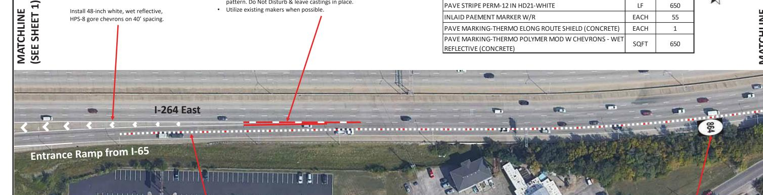
• Remove existing 6-inch white skip line starting 225' in advance of the end of the modified gore from I-65, heading east to KY 864.
