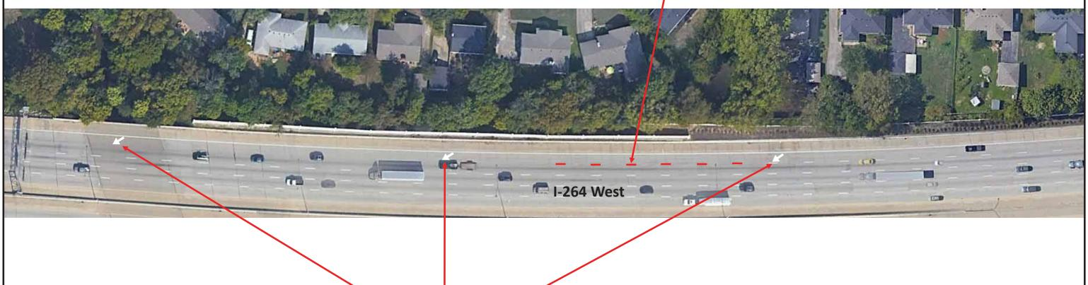
Install 4, wet reflective, HPS-8 lane reduction arrows on approximate 375' spacing. Install the last arrow 100' in advance (east of) the overhead sign truss. First arrow on previous sheet. If possible, avoid pavement joints with minor spacing adjustments.
