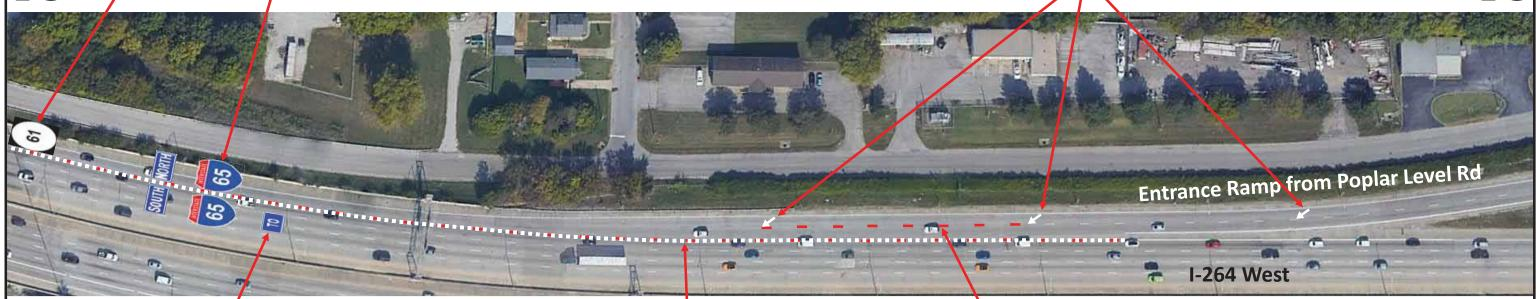
Install thermo "TO" approximately 40' in advance of the I-65 South shield. Adjust location as necessary to avoid damaged pavement and joints.
