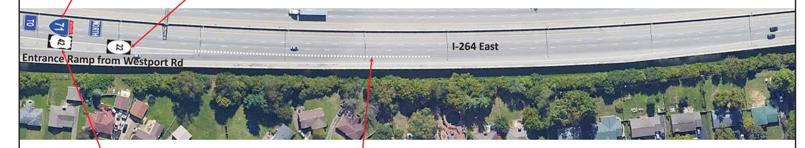
Install one US 42 thermo elongated route shield in the exit only lane approximately at the end of the barrier/sound wall at the entrance ramp from Westport Rd. Adjust location as necessary to avoid damaged pavement and joints.
