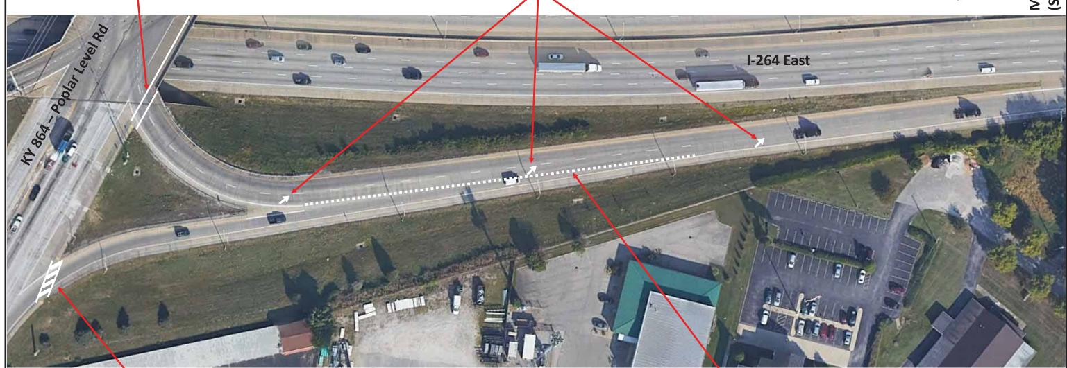
Install 6-inch white HPS-8 crosswalk stripes and 24-inch white HPS-8 bars with 24-inch gaps. Install bars parallel with the flow of traffic. Crosswalks to be 10' wide. Remove any edge lines within the limits of the crosswalks.
