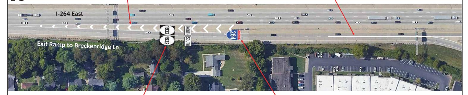
Install KY 1932 thermo elongated route shields in both exit lanes approximately 200' east of the exit ramp sign truss. Approximately 40' beyond the route shields, install a thermo "NORTH" in the left exit lane and "SOUTH" in the right exit lane. Adjust location as necessary to avoid damaged pavement and joints.
